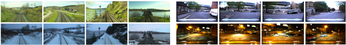
Fig. 9. Generalization results. Sample images (reference) of the Nordland summer (left-top) and Oxford RobotCar overcast traverses (right-top). Corresponding frames retrieved (query) using our FlyNet+CANN model from the Nordland winter (left-bottom) and Oxford RobotCar night traverses (right-bottom).
